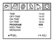
The TV set will switch to the preset channel when the **CH-TIME** elapses.
